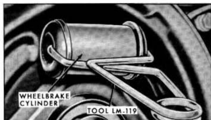
Fig. 2-10—Wheel Cylinder Clamp Installation—Typical—(61-CM-2002)
