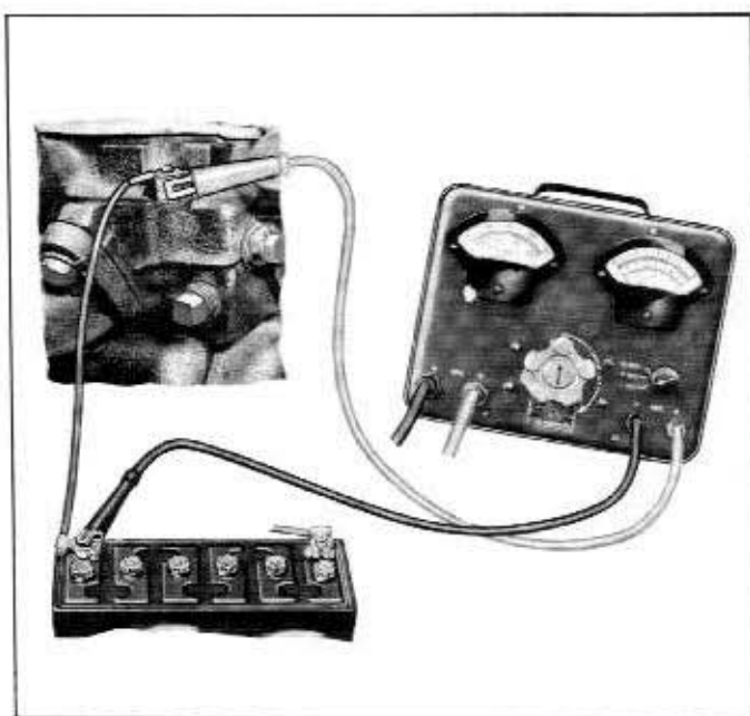
Fig. 9-24—Connections for Negative Battery Cable Resistance Test—(60C-7682)
