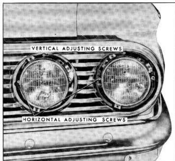
Fig. 10-1—Headlamp Beam Adjusting Screws—(61CM-7608)
