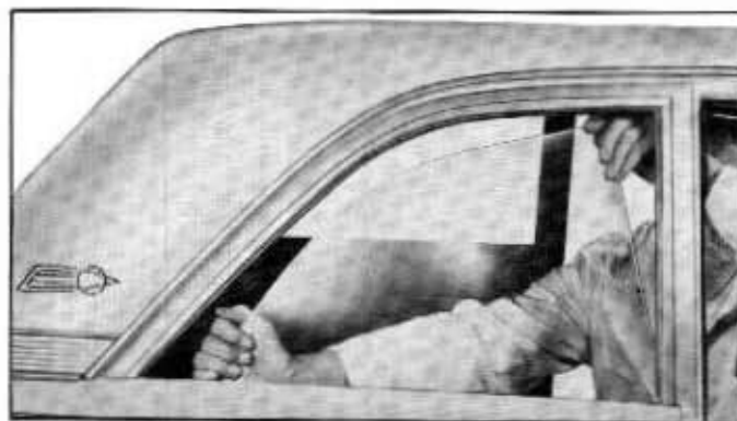
Fig. 13C-13—Quarter Window Glass Removal—(61CM-8010)
