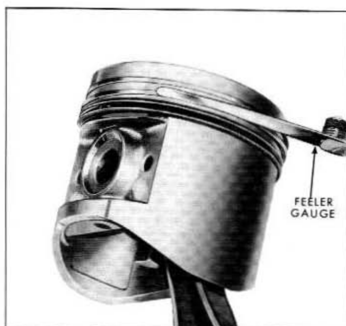
Fig. 6A-43—Checking Ring Side Clearance—Typical—(60C-5644)
