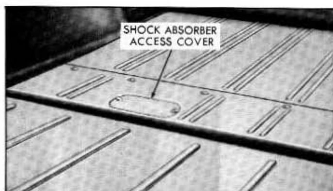
Fig. 4-3—Rear Shock Absorber Access Cover, Models 59A and 71A—(61CM-801)
