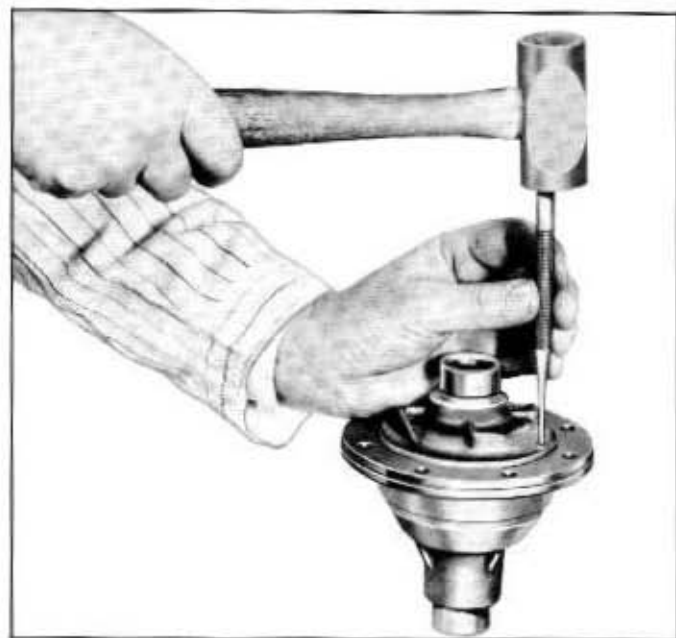
Fig. 4-21—Differential Pinion Shaft Retainer Removal—(60C-5212)
