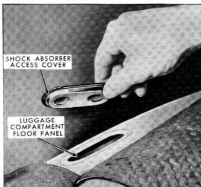
Fig. 4-2—Rear Shock Absorber Access Cover, Models 54A and 62A—(60C-802)
