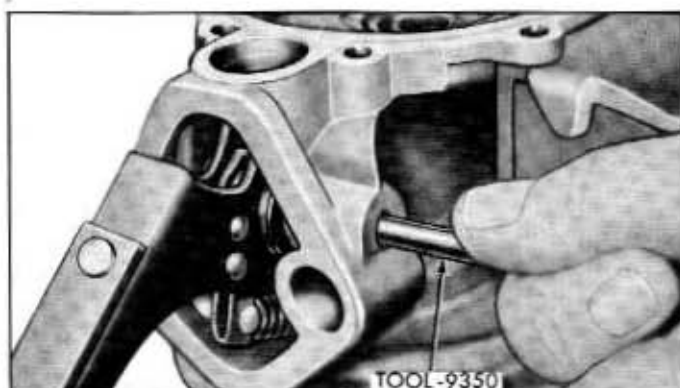
Fig. 8B-10—Holding Rocker Arm Assembly In Place—(61CM-6810)
