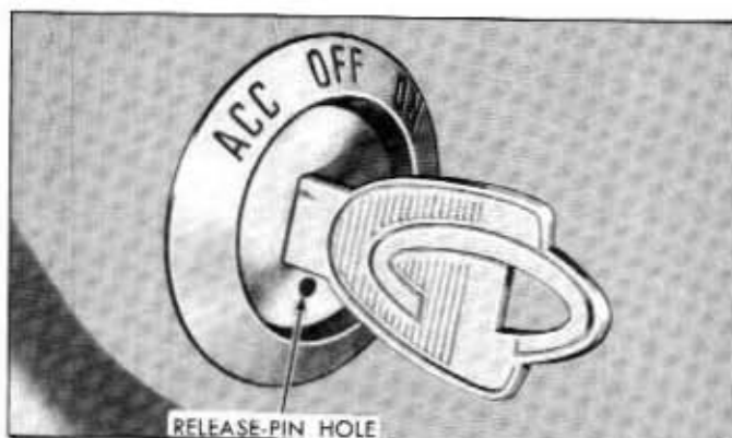
Fig. 10-9—Ignition Switch Removal—(60C-7634)
