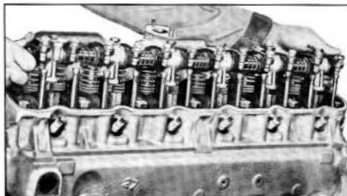
Fig. 6A-14—Valve Rocker Arm Shaft Removal—(60C-5614)
