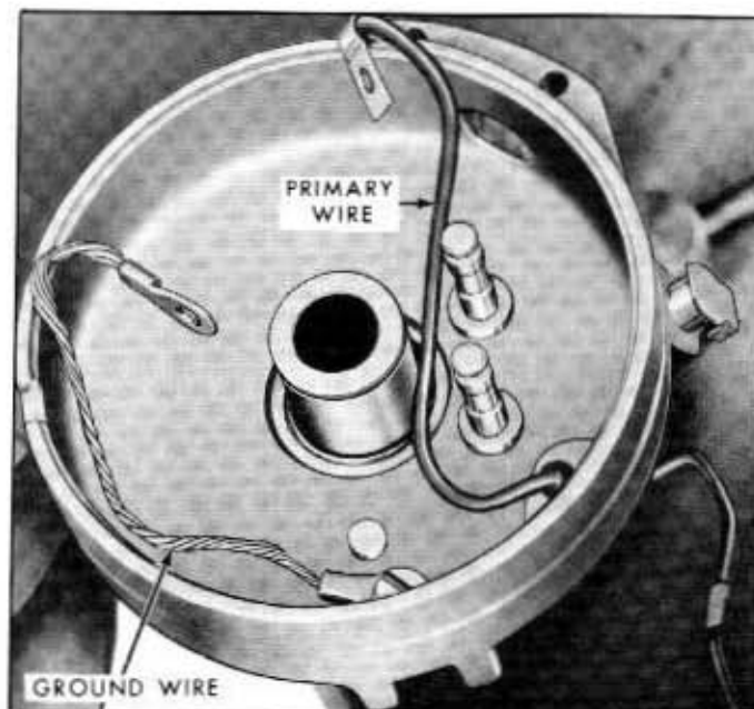
Fig. 9-66—Primary and Ground Wire Installation—(60C-7723)
