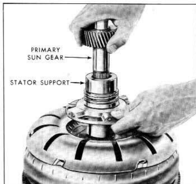
Fig. 7A-46—Stator to Turbine Interference Check—(60C-4446)
