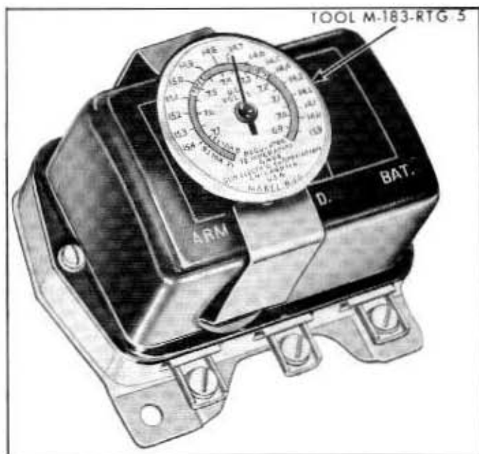
Fig. 9-19—Temperature Gauge for Voltage Setting—(8M-7781)
