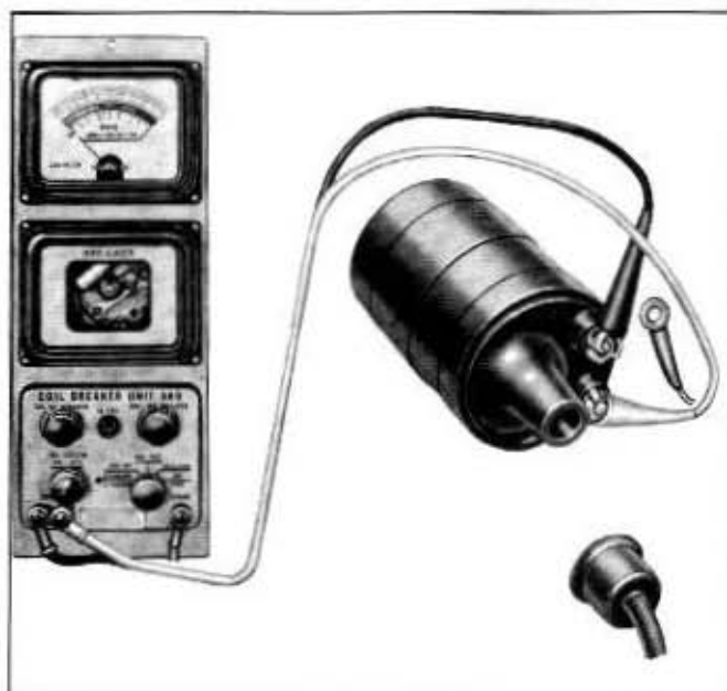
Fig. 9-50—Coil Capacity Test—(58L-419)
