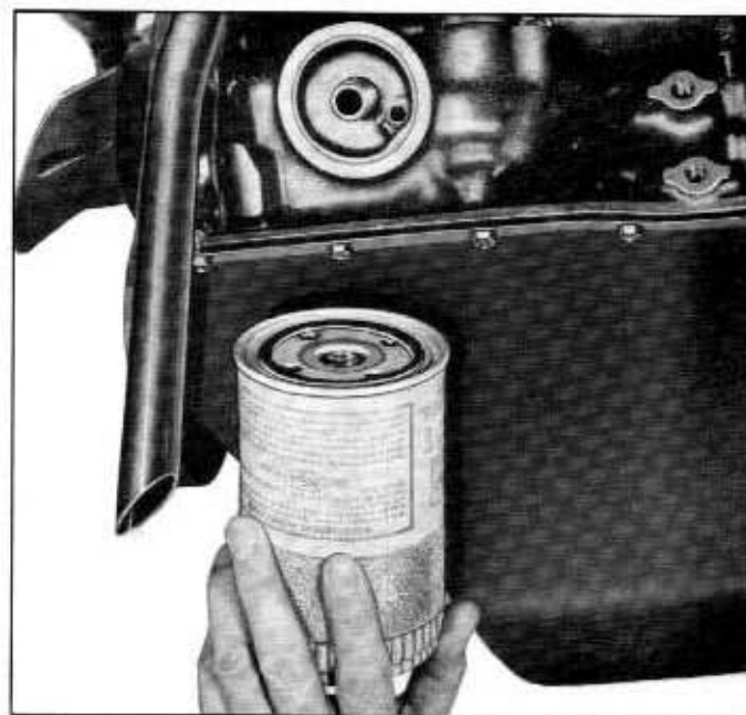
Fig. 6A-57—Oil Filter Installation—(60C-5657)
