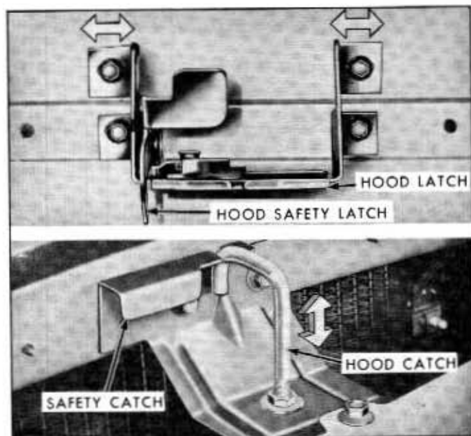
Fig. 13J-3—Hood Lock Adjustments—(60C-8006)
