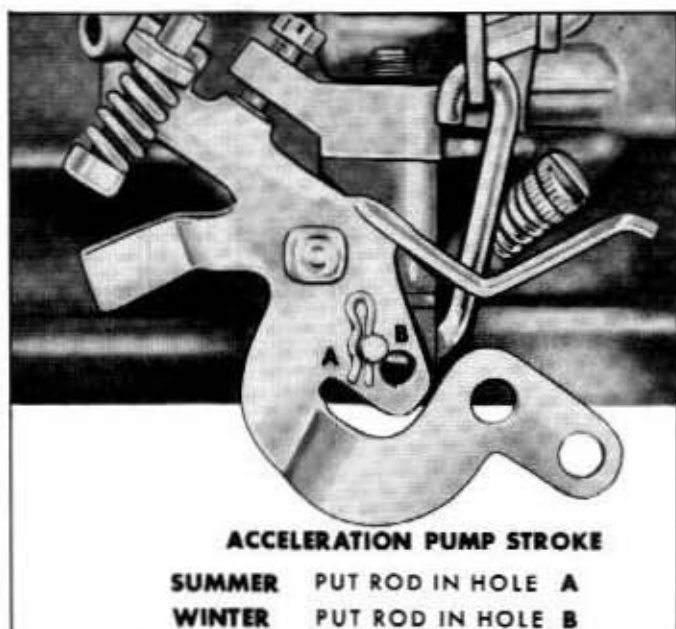
Fig. 8C-11—Accelerating Pump Stroke Adjustment—(61CM-6831)
