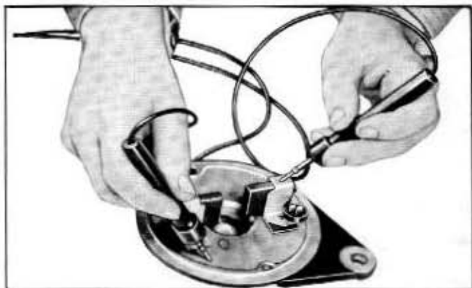
Fig. 9-12—Testing for Grounded Brush Holder—(60C-7671)
