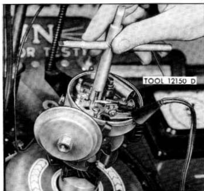
Fig. 9-56—Adjusting Point Alignment—(60C-7713)
