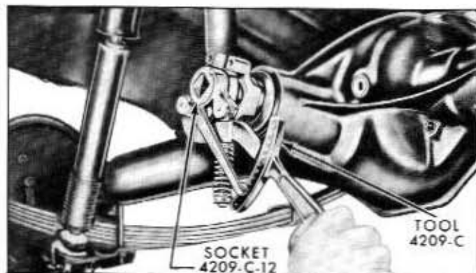
Fig. 4-29—Pinion Bearing Preload Check—(60C-5220)
