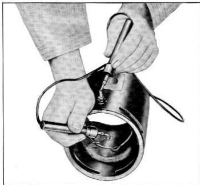
Fig. 9-10—Testing Field Coils for Open Circuit—(60C-7669)
