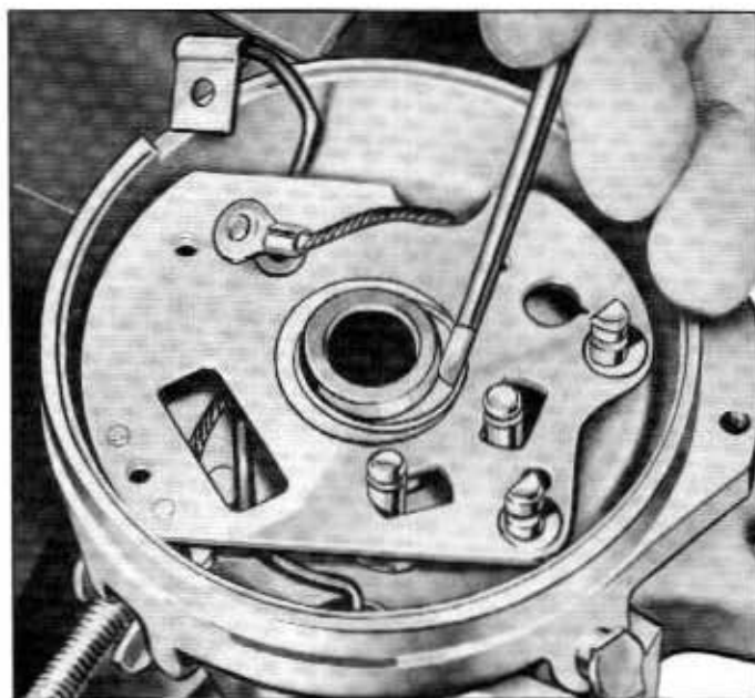
Fig. 9-62—Lock Ring Removal—(60C-7719)
